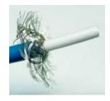
Open the braid carefully to sheath side, not to deform the braid by removing abt.30mm sheath. Remove the tape by making a nick all around of AL/PET Tape on x-point of braid foot by cutter, etc.
